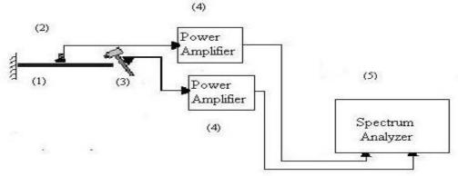
1- Cantilever beam, 2- Accelerometer, 3- Impact hammer with (piezoelectric cells),
